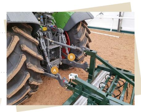
Reverse the tractor up to the grader and lift the tractor arms up to catch the tractor balls. Make sure the clips are in place to stop the balls coming out of the arms during grading.
